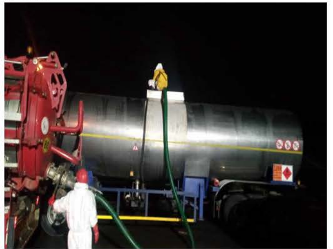
Super sucker offloading contaminated water into the road tanker.
