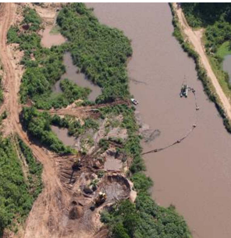
Various methods used to extract sand, including mechanical digging and dredging in an estuary (2019) Photo: Kierran Allen
